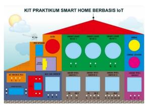
Fig. 1. Layout design of the trainer kit smart building
